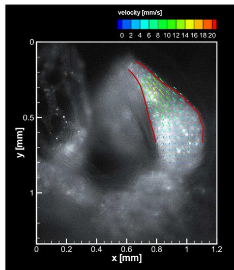
**Figure 3.** PIV measurement in the ventricle (left) and in the atrium (right) of a chicken embryo.
