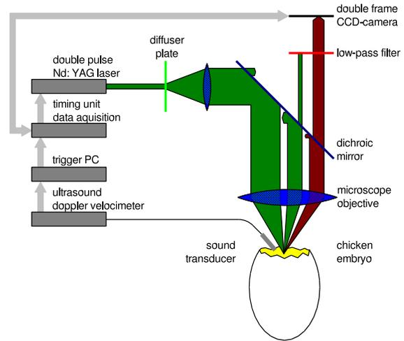
**Figure 2.** The  $\mu$ PIV set-up, using a fluorescence microscope.
