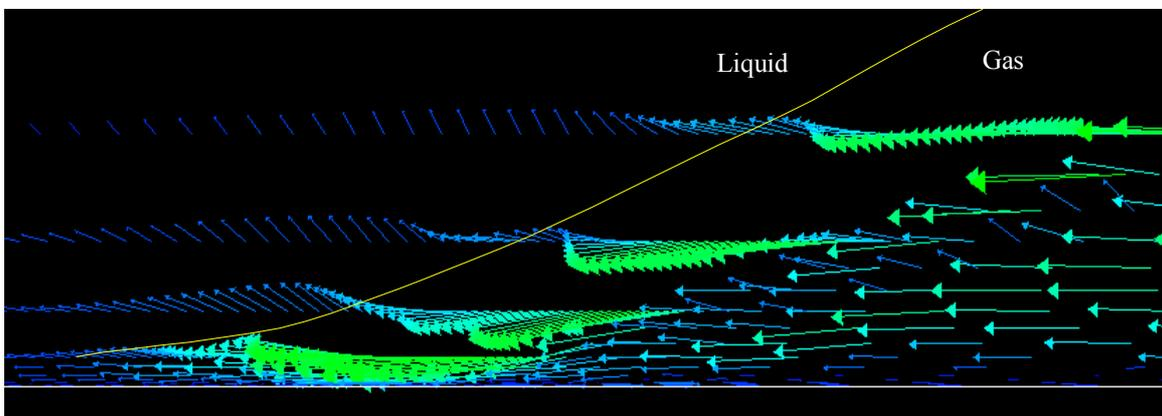
Figure 4: Velocity Vectors for liquid and gas jet system under normal operating conditions
