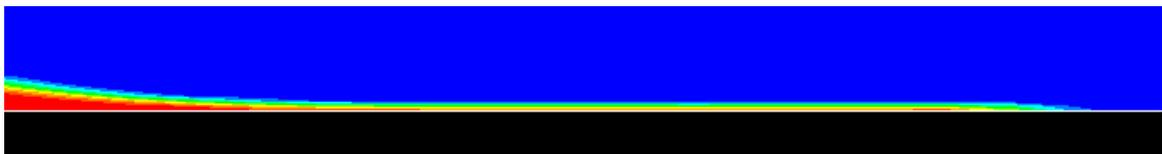
Figure 3: Liquid fraction contour of the residual liquid film left behind the liquid jet
