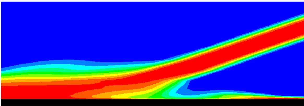
Figure 2: Magnified view of liquid jet with gas jet interaction under normal operating conditions
