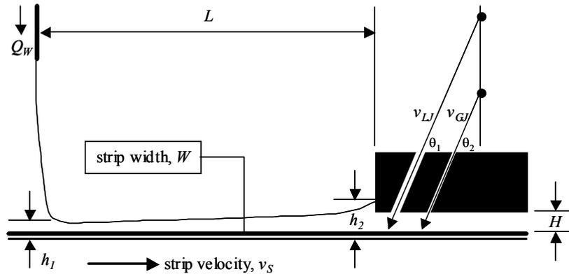
Figure 1: Basic Geometry for the Analytical Model
