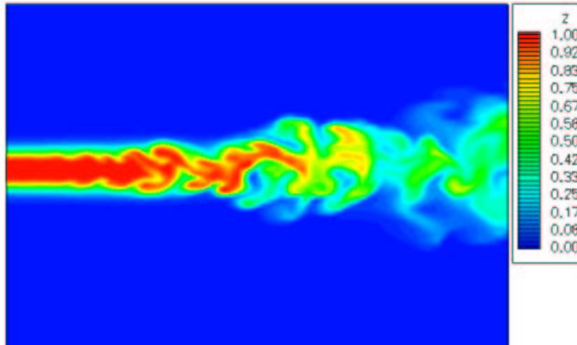
Figure 1. Mixture fraction contours in Sandia D flame.
