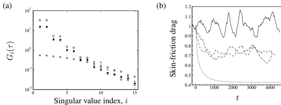
**Figure 1.** (a) Comparison of singular values for a wavenumber ( $k_x = 0, k_z = 6$ ):  $\circ$ , no control;  $\bullet$ , opposition control;  $\times$ , LQR control;  $\triangle$ , virtual flow. (b) Mean skin-friction drag history: —, no control; ---, opposition control, - · - · -, LQR control; ·····, virtual flow. Here,  $Re_\tau = 100$ .
