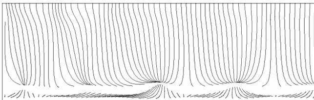
Fig.2 streamlines using the projected velocity near the upstream end wall ( $\Gamma = 6.55$ ) (left half plane,  $\Gamma = 6.55$ )
