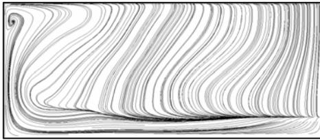
Fig.1 streamlines using the projected velocity near the upstream end wall ( $\Gamma = 4$ ) (left half plane,  $\Gamma = 4$ )
