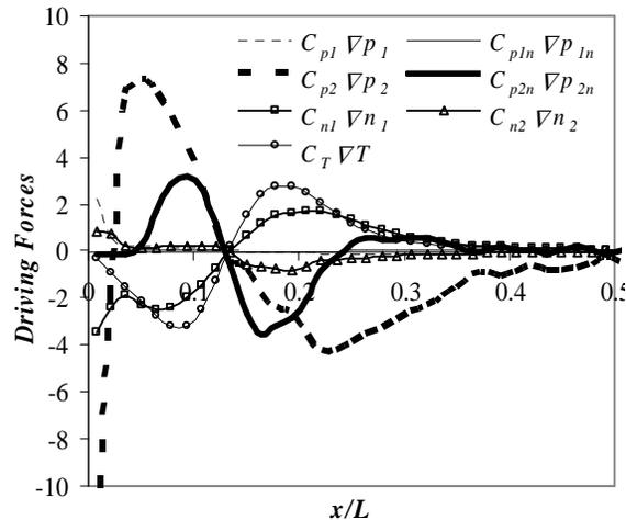
Figure 2. Driving forces for segregation using a form of Jenkins and Mancini [3] diffusion of velocity equation and simulation results. Relevant parameters:  $\phi = 0.1$ ,  $\phi_1/\phi_2 = 4.0$ ,  $d_1/d_2 = 2.0$ ,  $\rho_{p1}/\rho_{p2} = 8.0$ ,  $e = 0.9$ ,  $T_H/T_C = 10$ , and  $L/d_1 = 62.6$
