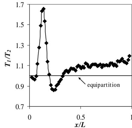
Figure 1. Granular temperature ratio of species 1 to species 2 ( $T_1/T_2$ ). Relevant parameters:  $\phi = 0.1$ ,  $\phi_1/\phi_2 = 4.0$ ,  $d_1/d_2 = 2.0$ ,  $\rho_{p1}/\rho_{p2} = 8.0$ ,  $e = 0.9$ ,  $T_H/T_C = 10$ , and  $L/d_1 = 62.6$
