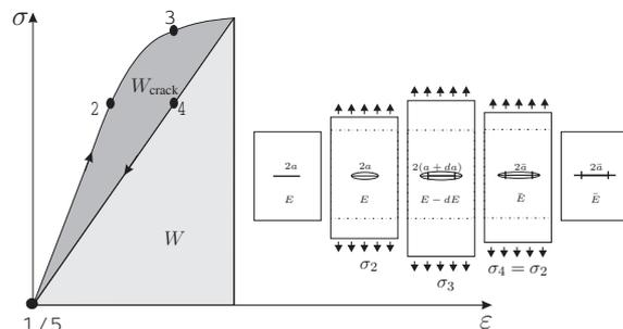
Fig. 1: The stress strain curve resulting from a growing (micro)-crack
