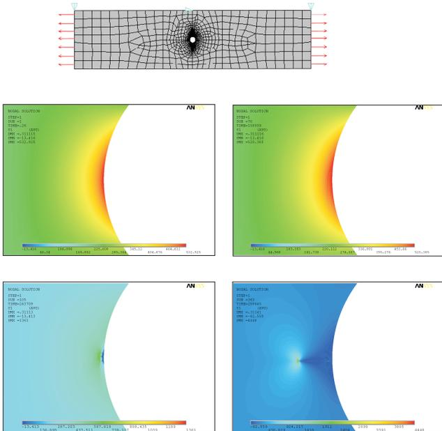
Fig. 4: The specimen and the evolution of stress state over lifetime
