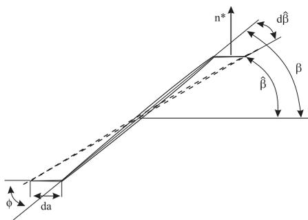
Fig. 2: The kinked and the replacement crack
