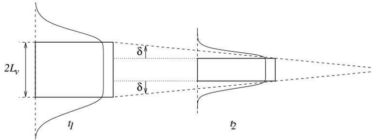
**Figure 3.** Schematic diagram of the two boundary layers during the slimdown regime.
