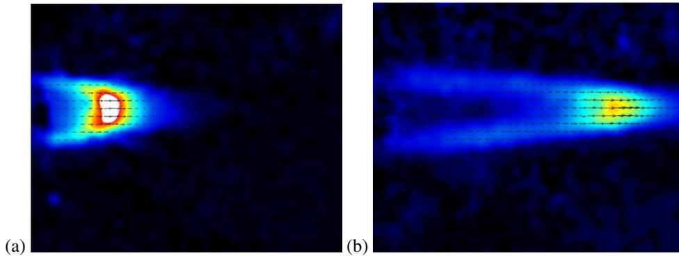
**Figure 2.** PIV measurements on a vertical cross-section through the dipole symmetry axis of the velocity modulus  $|V|$ . The initial instant immediately after the dipole has come out of the screen is shown in (a). In (b) the same frame 90 seconds later.
