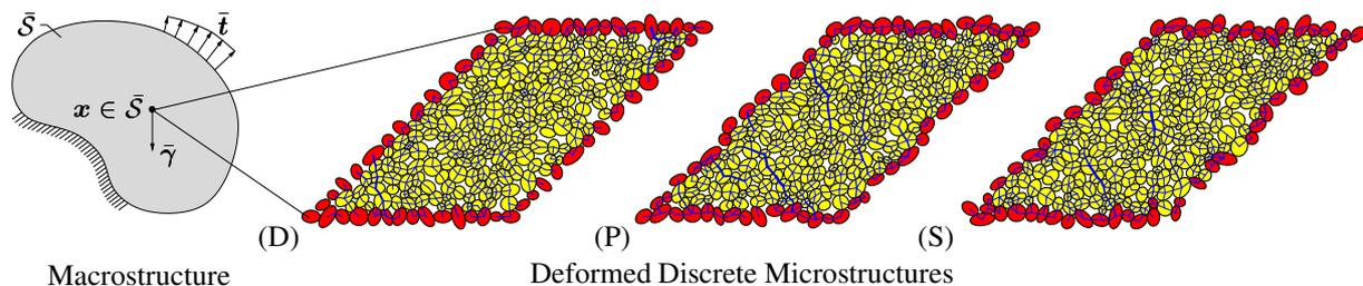
**Figure 1.** Deformed continuous macrostructure with a granular microstructure locally attached at a point  $\bar{x} \in \bar{S}$  under (D) linear deformations, (P) periodic displacements and (S) uniform traction constraints on the surface of the representative volume element.
