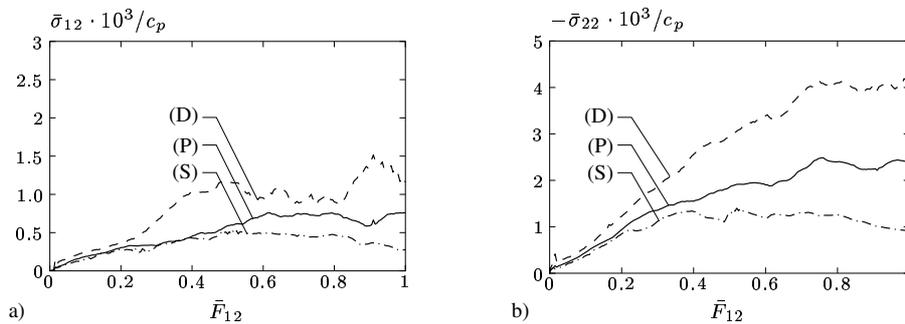
**Figure 2.** Homogenized a) shear stresses  $\bar{\sigma}_{12}$  and b) compressive stresses  $-\bar{\sigma}_{22}$  versus macroscopic shear deformation  $\bar{F}_{12}$  for the three types of boundary conditions (D) linear displacements, (P) periodic deformations and (S) uniform tractions on the surface. The simulation was carried out with a granular plane microstructure of 256 elliptically–shaped particles.
