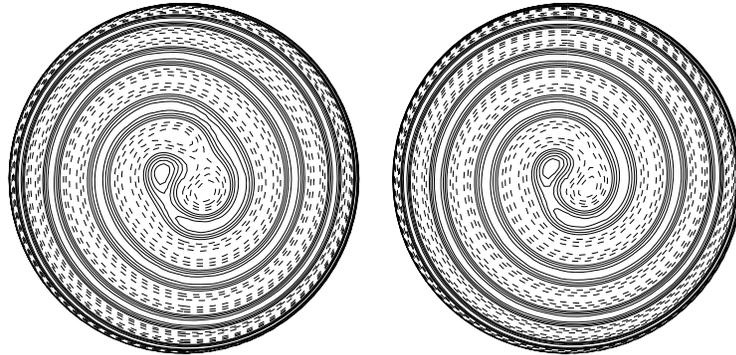
**Figure 1.** Contours of radial flow  $u_r$  at the middle surface of the spherical shell for  $\epsilon = (R/R_c) - 1 = 0.28$  ( $R_c = 1712$ ) and  $Pr = 7.0$ . Dashed contours indicate radially inward flow  $u_r < 0$  and solid contours correspond to radially outward flow  $u_r > 0$ . The top (middle) panel shows the contours viewed from the north (south) pole.
