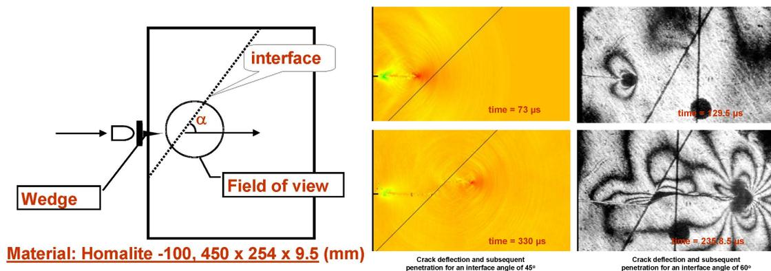
**Figure 1.** Sketch of the experimental set up (left): a pre-notched homalite plate with an inclined interface under a dynamic wedge-loading mechanism, and qualitative comparison of simulation and experiment (right).
