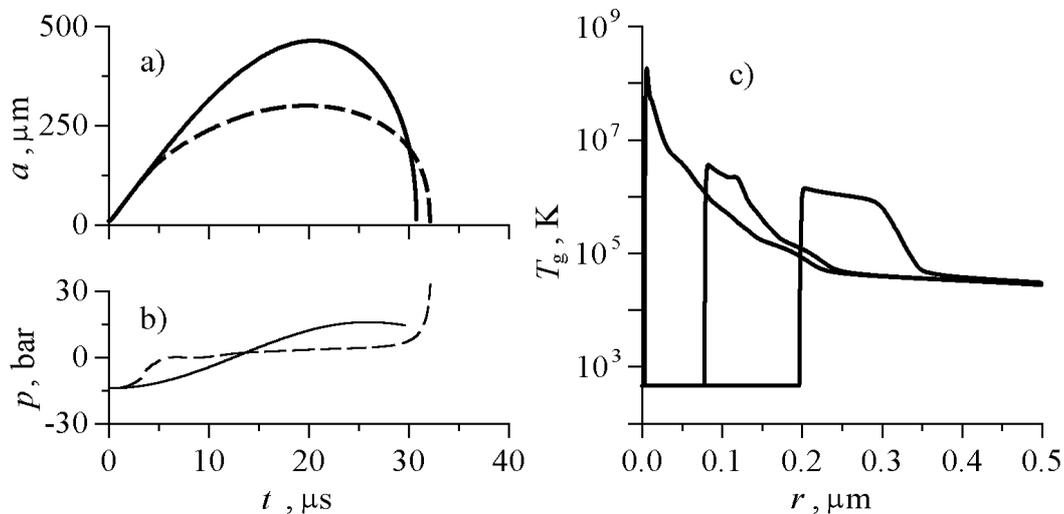
**Figure 1.** Bubble radius (a) and liquid pressure (b) evolution in time. Solid line – single bubble, dashed line – bubble in 20-bubbles cluster. Focusing of a shock wave near the bubble center (c).
