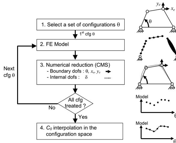
**Figure 1.** Basic principle of the reduction method. Illustration: a flexible four bar system, where the effector motion  $(x_e, y_e)$  is controlled at the joint angle  $\theta$ . The configuration space is 1-dimensional.
