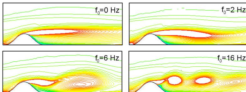
Fig.2. Instantaneous vorticity fields behind the hill for different frequency of incident oscillation ( $t/T_0=0.25$ ).
