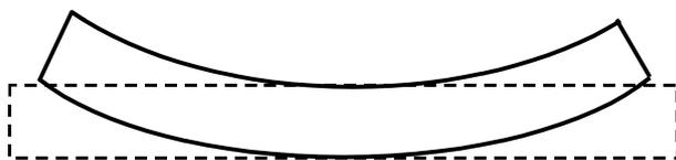
Fig. 1. The scheme of plastic bending of chalcogenides (HgSe, Hg<sub>1-x</sub>Cd<sub>x</sub>Se, HgSe<sub>1-x</sub>S<sub>x</sub>) samples investigated after applying of hydrostatic pressure.
