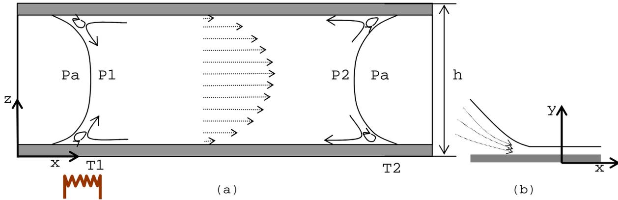
**Figure 1:** (a) A Schematic illustration of the studied system of a liquid drop moving in micro-channel with a rectangular cross section. The flow inside the micro-channel is induced by thermocapillary motion. (b) A sink-like flow illustration at the corner of the micro-channel as a result of a pre-wetting condition.
