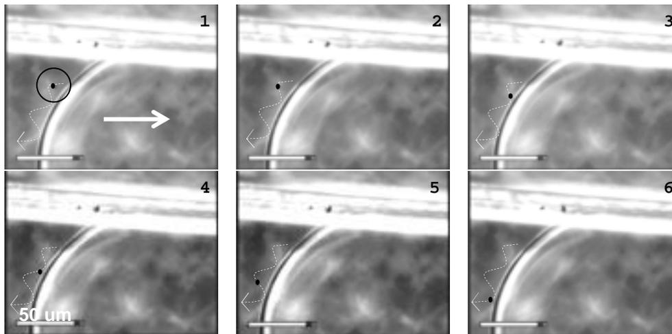
**Figure 3:** A series of pictures taken in the vicinity of the dynamic contact line during the droplet movement. The center of gravity of a nanowire (marked with a black dot) is moving along a non-closed spirally shaped streamline.
