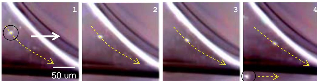
**Figure 4:** A series of pictures taken in the vicinity of the dynamic contact line during the droplet movement where a pre-wetting condition of the channel exists. The centers of gravity of the nanowires (marked with a white dot) are moving along sink-like flow streamlines.
