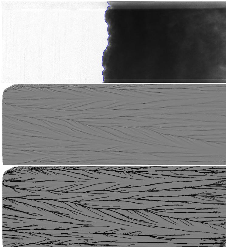
**Figure 1.** a) Contour mapping. The motion of the gravity current in all figures is right to left. b) Curvature of first arrival time field. Black corresponds to curvatures less than -2 (inverse pixels), white to great than +2, and the intensity is linear in between. c) Position of clefts superimposed on curvature picture
