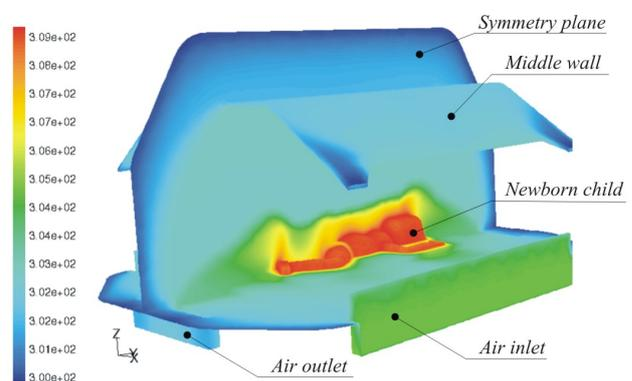
**Figure 2.** Perspective view of the temperature field.
