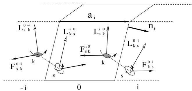
Figure 2. A cell of a crystal. Discrete model
