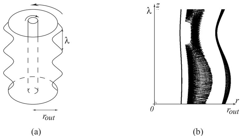
**Figure 1.** (a) The flow setup. (b) Projection of three streamlines on the  $(r, z)$  plane (periodic boundary conditions in  $z$  were imposed). The right and left streamlines are regular, the middle one is chaotic.
