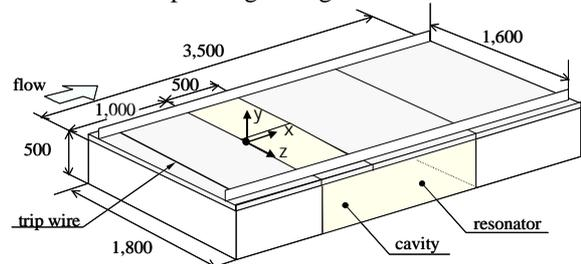
Fig.2 The model with a cavity (RTRI)
