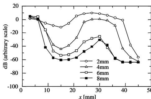
Fig.5 Variation of peak level with plates of different vertical lengths and  $x$  locations (IFS)
