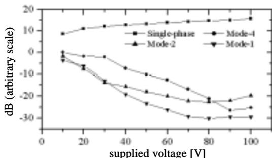
Fig. 3 Noise suppression effect of bimorph actuators (IFS)
