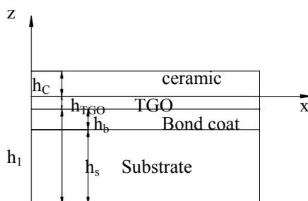
Fig.1 Cross-section of thermal barrier ceramic coating system
