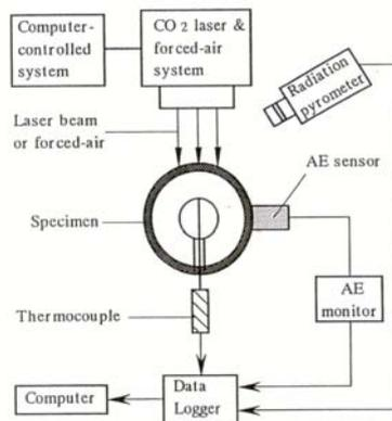
Fig.4 Schematic of the experimental setup for CO<sub>2</sub> laser heating method
