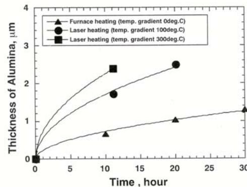
Fig.5 The effect of temperature gradient on the thickness of thermal growth oxidation, i.e., alumina
