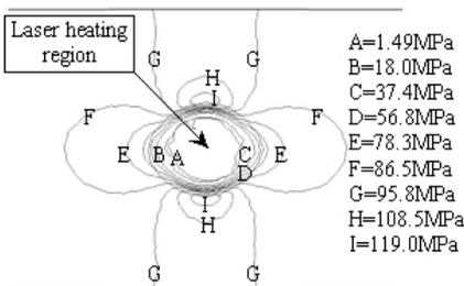
Fig.5 The stress field,  $\sigma_{xx}$ , on the laser heating surface
