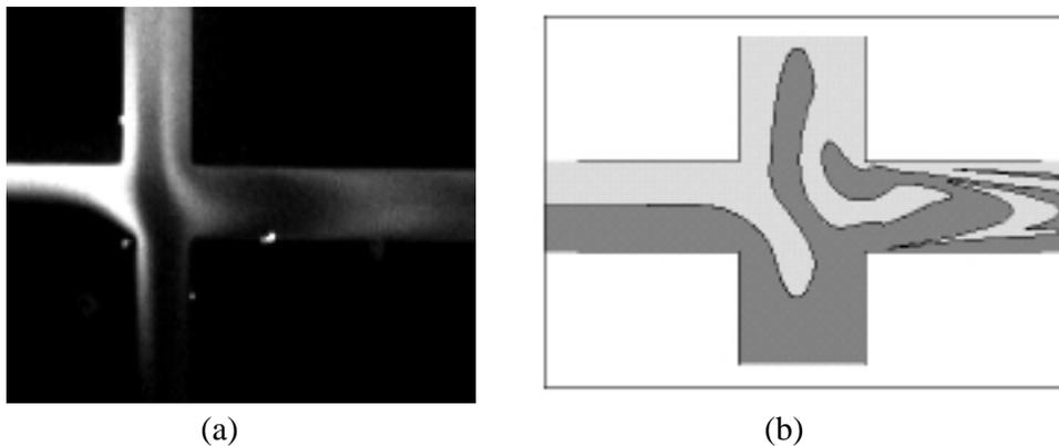
Figure 3: Shape of the interface at the cross-channel intersection a) experimental b) numerical simulation. Experiment agrees with numerical simulations.
