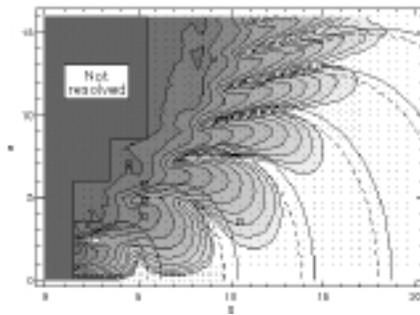
Figure 2: Contour-plot showing the amount of mixing as a function of the non-dimensional amplitude  $\omega$  and frequency  $\Omega$ , where darker gray means better mixing and visa versa. The resonances are the light spikes entering the darker region, and their theoretical predictions are the solid thick curves.
