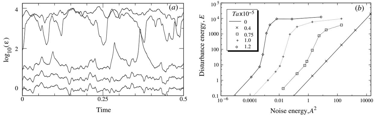
**Figure 1.** Transient disturbance energy at a variable noise amplitude,  $Ta = 10^5$  (a) and the response function (b).
