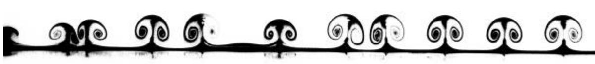
Figure 1. 'Mushroom' vortices along the widest part of the cylinder generated by oscillatory motion in the direction normal to the page.
