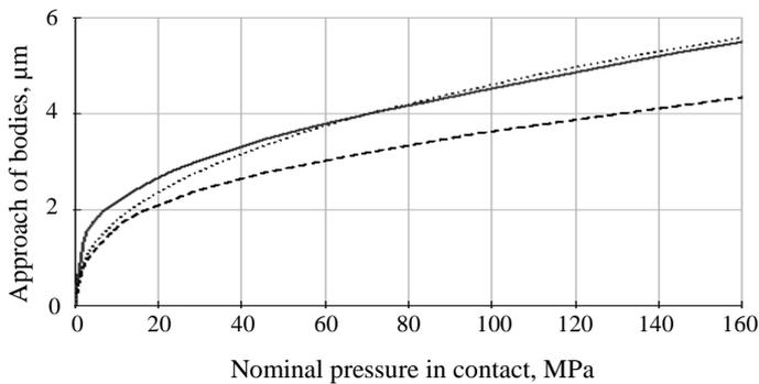
Figure 2. Approach of bodies with rough surfaces
