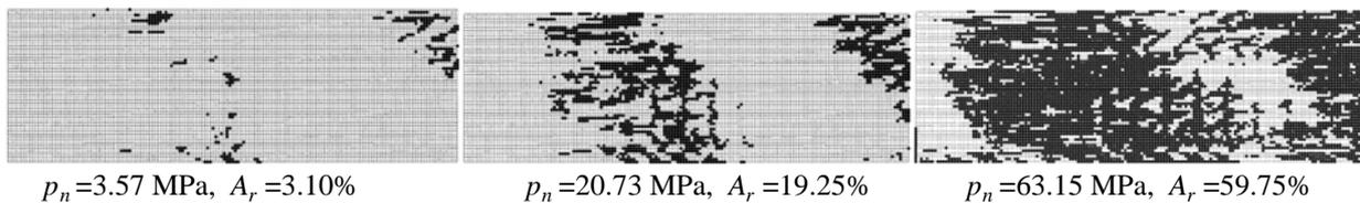
Figure 3. Real contact area during load increment
