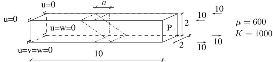
Figure 2: Model of cantilever beam
