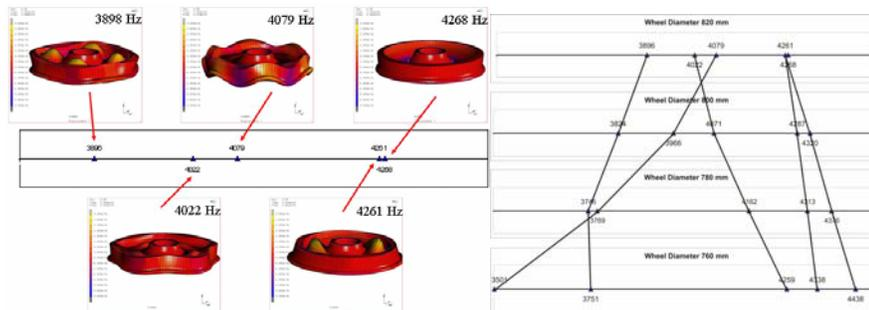
Figure 2: Left: Eigenforms of new wheels in the area of 4000 Hz. Right: Eigenfrequencies versus wheel radius for different eigenforms.
