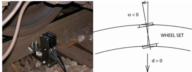
Figure 1: Setup for the measurement of striking angle ( $\alpha$ ) and lateral displacement ( $d$ ). The setup consists of two high definition lasers attached directly on the flange of rail.
