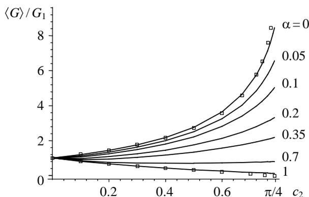
Fig. 1. Effective shear modulus  $\langle G \rangle$ ;  $G_2/G_1 = 20$ .
