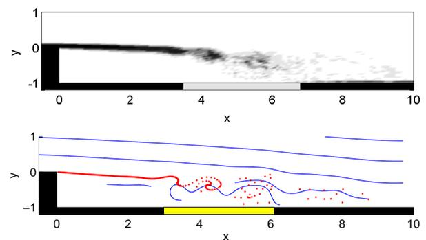
Fig. 3: Numerical simulation (top) and low-dimensional vortex model with  $\approx 300$  vortices (bottom) of the flow around a backward-facing step at  $Re_h = 4000$ . The top figure illustrates the vorticity distribution of a snapshot. The figure at the bottom indicates vortex locations by red dots. Regions of upstream velocity close to the wall are marked by grey bars.
