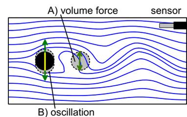
**Fig. 1:** Streamlines of the von Kármán vortex street in the wake of a circular cylinder at  $Re = 100$ . Two different actuators are investigated: A) a local volume force, and B) oscillations of the cylinder. The state of the flow is monitored by a single hotwire probe.
