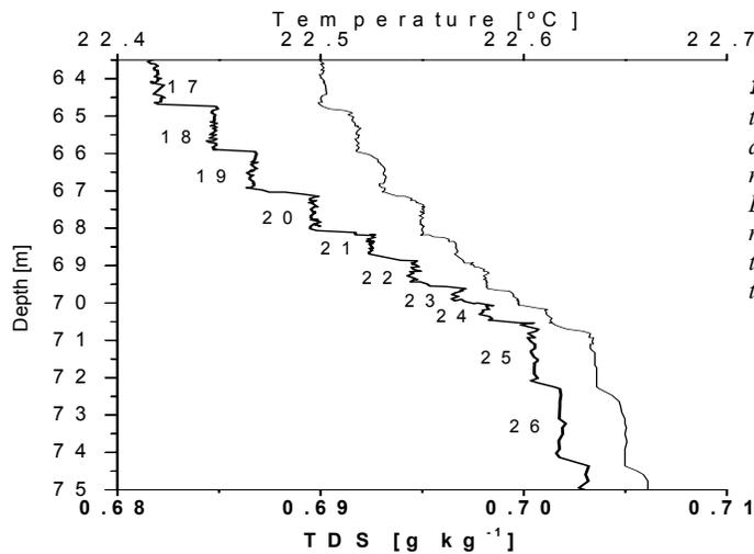
**Figure:** Details of an 11-m long section from the profiles of temperature (thin line) and total dissolved solids (TDS) (thick line with layer numbers) measured on 8 December 2002 in Lake Nyos. The observed convectively well-mixed layers are numbered from the top. Note that the interfaces are much steeper for temperature than for TDS.
