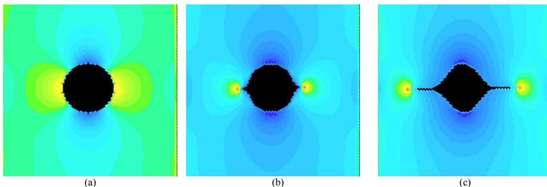
Figure 3. Evolution of a void in an elastically stressed body for  $K_0=1$ ,  $\alpha=6000$  and an applied strain of 0.3%. (a) The plate is under uniaxial tension in the vertical direction. (b) Material flows over the surface of the void from areas of high elastic energy (red) to areas of low elastic energy (blue) causing small notches to appear on the side of the void, (c) the stress is raised at the notch tips causing them to grow into crack-like features.
