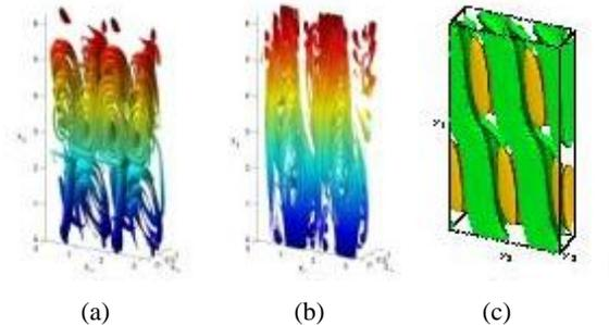
Fig. 2. Flow field associated with 4th mode (a) streamtube without mean velocity. (b) streamtube with mean velocity. (c) temperature isosurface.
