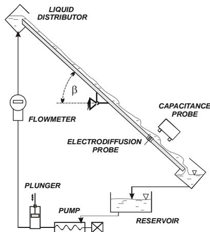
Fig.1 Experimental set-up
