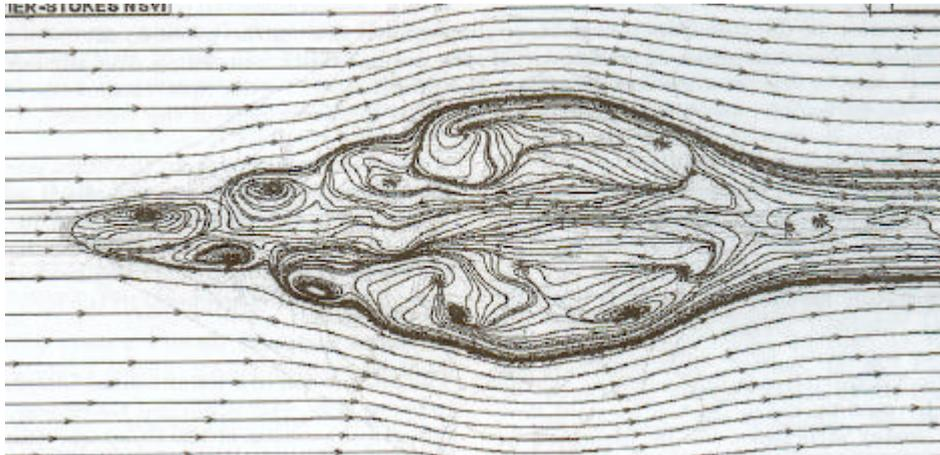
Fig. 1: Streamlines for normal shock-vortex interaction for  $Ma_{\infty} = 1.6$  and  $Re_{\infty} = 1.5 \cdot 10^3$ ; obtained with solution of Navier-Stokes equations.
