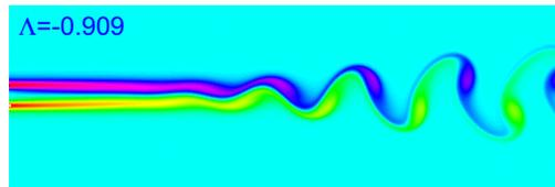
**Figure 2.** Global Mode of the nonparallel wake obtained for a Reynolds number  $Re = 800$  for  $\Lambda = -0.909$ , i.e. when the inlet flow is everywhere positive. This Reynolds number is well above the absolute instability threshold  $Re_A \sim 125$  for this particular value of  $\Lambda$ . The computation box is 16.8 large and 51.2 long, the wake width being unity.
