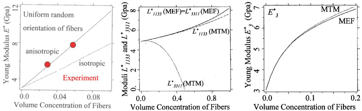
Fig. 1. Modulus  $E^*$  (GPa) vs  $c$     Fig. 2.  $L^*_{1133}$  and  $L^*_{3311}$  (GPa) vs  $c$     Fig. 3.  $E^*_3$  (GPa) vs  $c$
