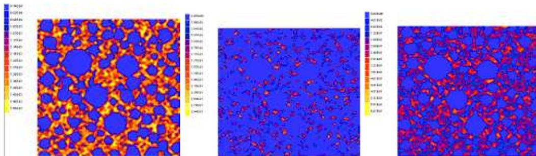
Figure 1. Simulation results for the damage calculus in a HSC under thermal loads (thermal strain fields, damage at 50°C, 120°C)
