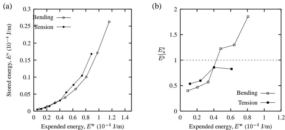
**Figure 2.** Energy storage under two deformation states, tension and bending. (a) Stored energy,  $E^s$ , versus expended energy,  $E^w$ . (b) Ratio of stored energy in the unloaded state,  $E_u^s$ , to  $E^s$  versus  $E^w$ .
