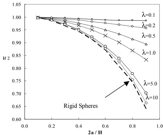
**Figure 1.** Translational velocities along the channel ( $u_2$ ) of spherical drops for various viscosity ratios as a function of relative drop size,  $2a/H$ , where  $a$  is the drop radius. The dashed line represents data for rigid spheres. The corresponding viscosity ratios are indicated above the curves.
