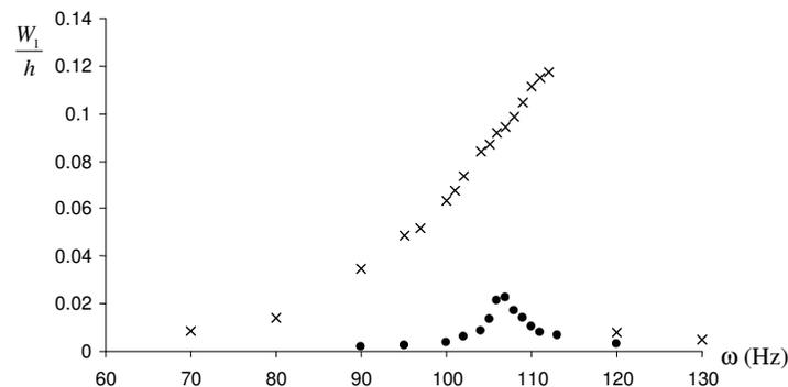
Figure 1. Normalized displacement amplitude, 1<sup>o</sup> harmonic, excitations with amplitudes: o 100 mN, x 400 mN.
