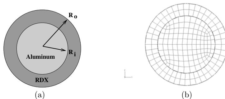
Figure 1: Schematic of (a) an explosively coated aluminum grain and (b) the computational grid within a grain used for the representative simulation.
