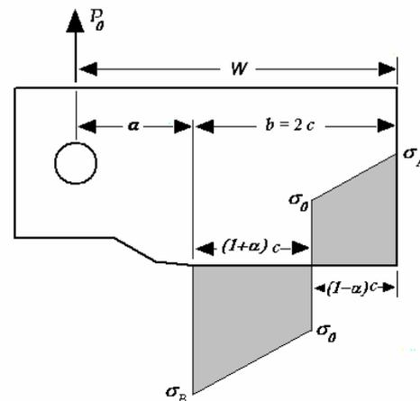
Figure1: CT specimen and stress distribution in remaining portion.
