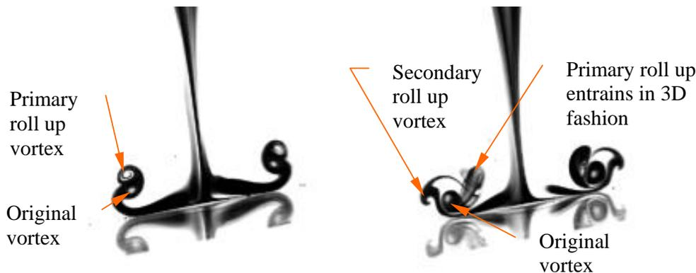
**Figure 1: Flow visualization using Laser Induced Fluorescence in the center plane of a vortex ring impinging perpendicular onto a wall. The light sheet is 4 mm thick and the diameter of the original vortex torus ca 50 mm wide. Two instances in time are shown. Left image is shortly before 3D breakdown; right image is at the instant of the 3D entrainment of the primary roll up vortex into the original vortex.**
