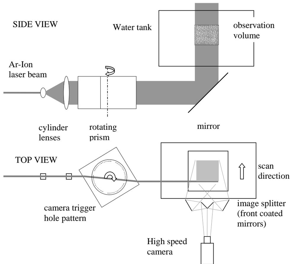
**Figure 2: Optical setup of the scanning PTV system used to increase the particle density in the observation volume. The light sheet undergoes parallel displacement depending on the rotation angle of the prism.**
