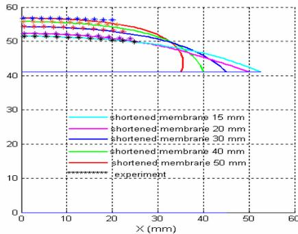
Fig.1 The deformed profiles of cylindrical membrane subjected to inner pressure  $p=0.5\text{MPa}$
