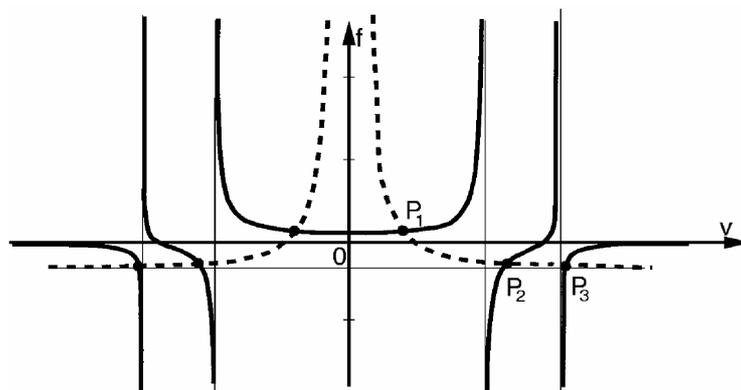
Fig. 2. Wave velocities in conventional track for the case when both rails vibrate “out of phase” and rails – sleepers vibrate “in phase”.
