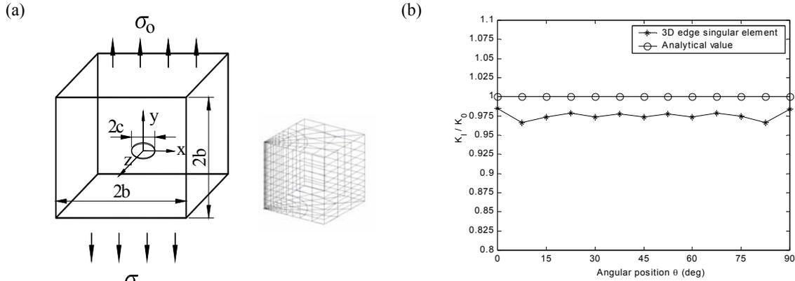
Figure 1: (a) Penny-shaped crack in homogeneous medium and the one-eighth model mesh. (b) Magnitude of stress intensity factor along crack front.
