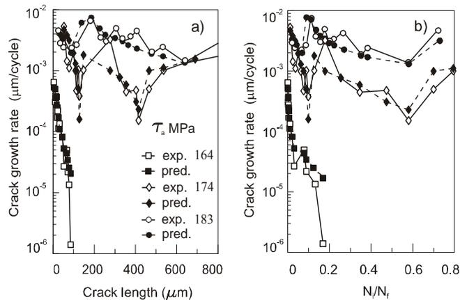
Fig. 1. Experimental and predicted plots of crack growth rate versus crack length and stress ratio  $N_i/N_f$
