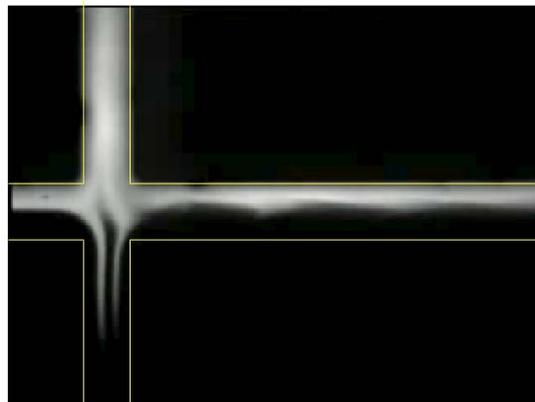
**Figure 2 :** In this particular case, the interface is strongly perturbed in the active zone, but returns straight as it leaves it. This is the “resonance” state. This state may be used produce efficient extraction of particles of
