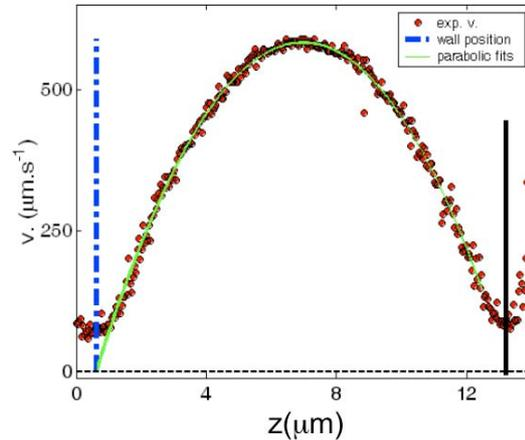
**Figure 1 :** Example of a velocity profile, obtained by using PIV, in a 12  $\mu\text{m}$  deep microchannel (red disks). The green line is a best fit, providing a slip length equal to  $-35 \pm 100 \text{nm}$ . The “foots” of the profile, within the first 400 nm close to the walls, are due to experimental errors. The data located within 400 nm is discarded in the best fit procedure.
