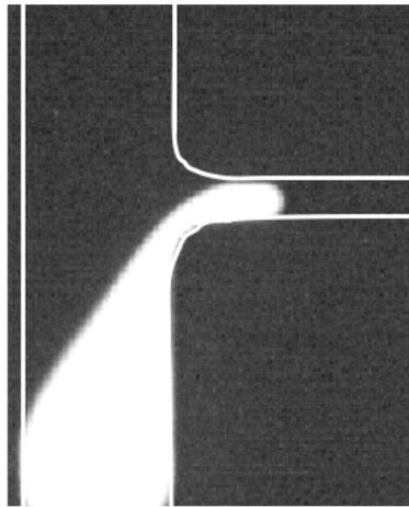
**Figure 3 :** Formation of a filament prior to drop break-up. The water drop (labeled with fluorescein, thus appearing as white on the picture) which is moving downwards will further split into two parts, one in the derivation channel, and the other in the main channel.
